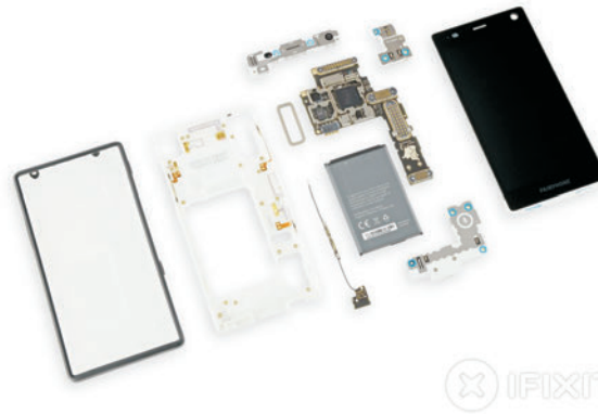
Disassembled Fairphone 2; (C) by iFixit GmbH
